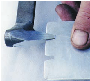
Check against nail or use a guide. This one is made from aluminum.
