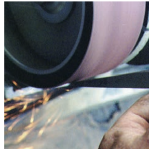
Pritchel with broken tip. Grind end flat. Grind to desired dimension. Use this approach to the wheel for aggressive stock removal.
