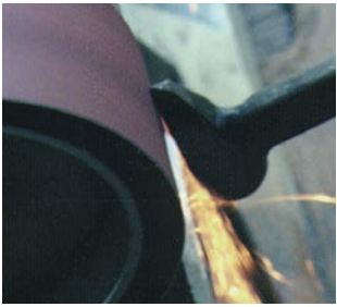
Grind back to desired nail dimension.
